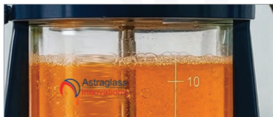
Live camera view with automated foam detection.
