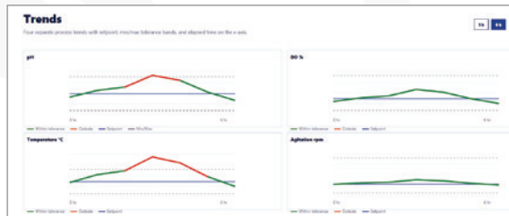
Real-time process trends with setpoint and tolerance bands.
